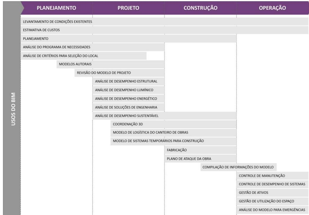
FIGURA 6:USOS BIM (ADAPTADO DE [HTTPS://BIM.PSU.EDU/USES/](https://bim.psu.edu/uses/))
