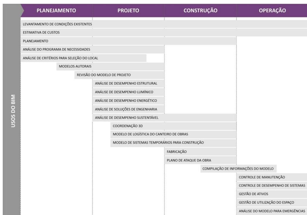
FIGURA 6: USOS BIM (ADAPTADO DE [HTTPS://BIM.PSU.EDU/USES/](https://bim.psu.edu/uses/))
